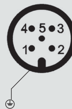
Circular connector M12 x 1, 5-pin
